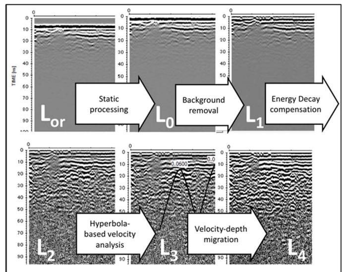
**Figure 3** Processing steps of the GPR signal
