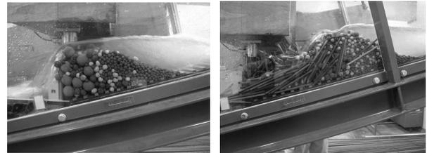
(c)  $K_w=0\%$ , -側面(d)  $K_w=20\%$ , -側面写真-1 土石流捕捉状況の一例(勾配15°,  $W/d_{95}=1.0$ )
